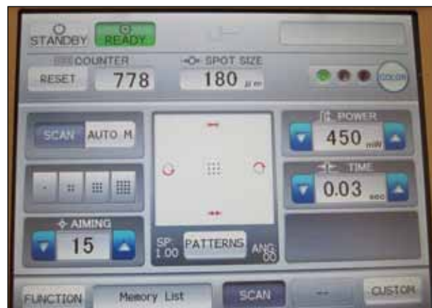
Figure 3. All laser parameters can be rapidly adjusted from the touch screen console.
